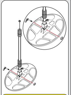
After placing the shaft on the coil as shown in the picture, insert the fastening screw through the hole and tighten it using the wingnut.
