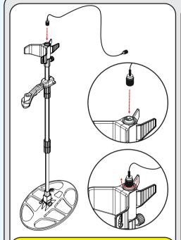
Insert the end connector on either end of the system connection cable into the socket on the handle and tighten securely.
