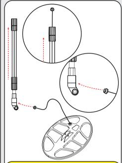
Insert the coil cable into the shaft. Do not extend the shaft prior to this step! Pull the cable out from the other end of the shaft.
