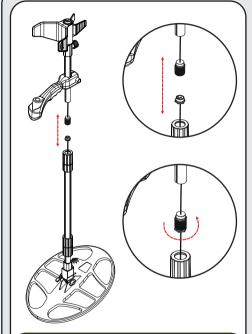
Connect the end connector on the search coil cable with the connector underneath the handle and tighten.
