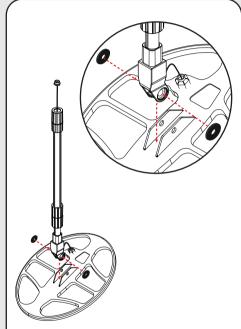
Place the washers into the openings on both sides at the end of the extension shaft.
