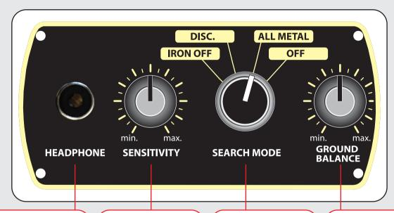
Headphone Input: To better hear the sounds produced by the device, connect the headphones to the system box. Sensitivity Setting: Is the depth setting of the device. For details please see page 17. Search Mode Knob: Is used to select the search mode as well as turning on/off the device. Ground Balance Knob: Is used to eliminate ground noise. For details please see page 18.
