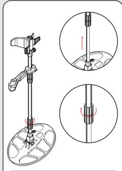
To adjust the height of the device, loosen the twist lock on the shaft. After adjusting the shaft length to your height, re-tighten.
