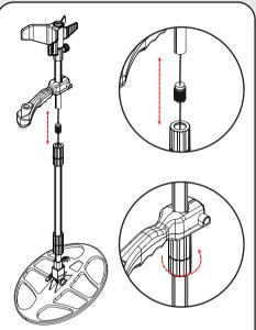
Insert the shaft in its socket underneath the handle and start rotating the twist lock. As you rotate the twist lock it will slide down. Before rotating the twist lock all the way, push the shaft up again making sure that it is in place and secure it by tightening the twist lock.
